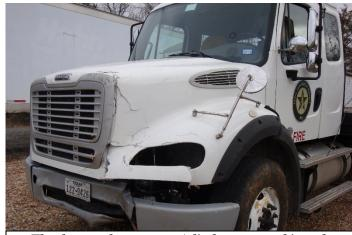
The damaged transport. A limb penetrated into the engine compartment causing damage
